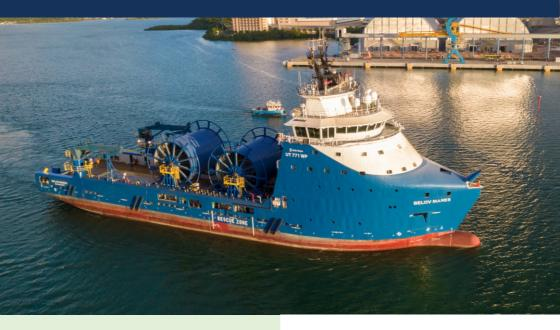
This OTSV is a Rolls-Royce design UT771 WP is a medium-sized offshore transfer supply vessel which undertakes supply duties between land bases and offshore installations. The model is designed for diesel electric medium or high-speed machinery and azipull propulsion system. The cargo deck area with two cranes, well protected and a deckload of 10 t/m<sup>2</sup>.
