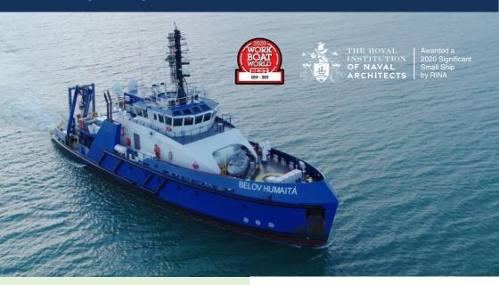
DSV designed by Robert Allan – Naval Architects and Marine Engineers (RAL). First brazilian diesel-electric diving support vessel. The DP-2 rated vessel is fitted with air diving capabilities, a light work-class ROV and knuckle-boom crane to allow effective offshore operations. The propulsion includes three main waterjets and three tunnel thrusters, which allow safe diving conditions while divers are near the surface.
