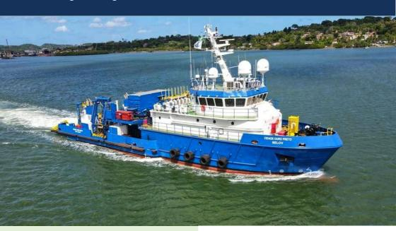
This DSV, designed by INACE – Indústria Naval do Ceará, is diesel powered DP-2 rated vessel, fitted with air diving capabilities, a light work-class ROV and knuckle-boom crane to allow effective offshore operations. The propulsion includes three main waterjets and two tunnel thrusters, which allow safe diving conditions while divers are near the surface.
